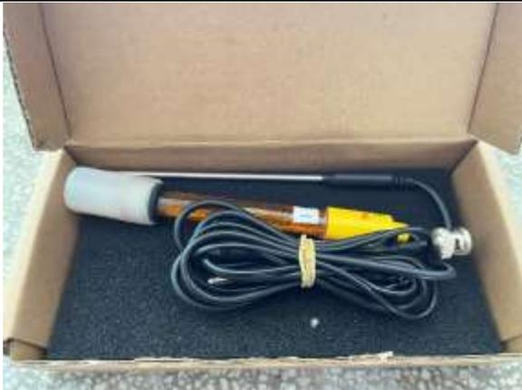
A photograph showing a pH electrode with a white handle and a yellow tip, connected to a blue cable. The electrode and cable are resting on a black foam pad inside an open cardboard box.                                                                         |
